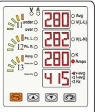
Page 1: Displays Amps L1, L2,L3 & Average Voltage ( L-L)
